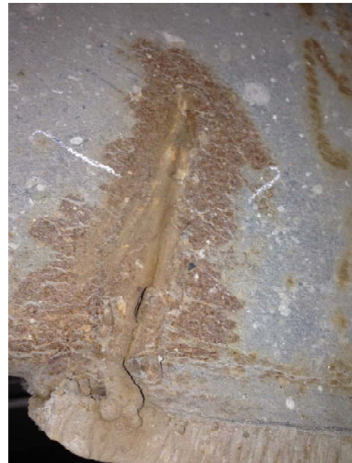
Cracked frame found on dump truck taken out of service, Feb. 25.
