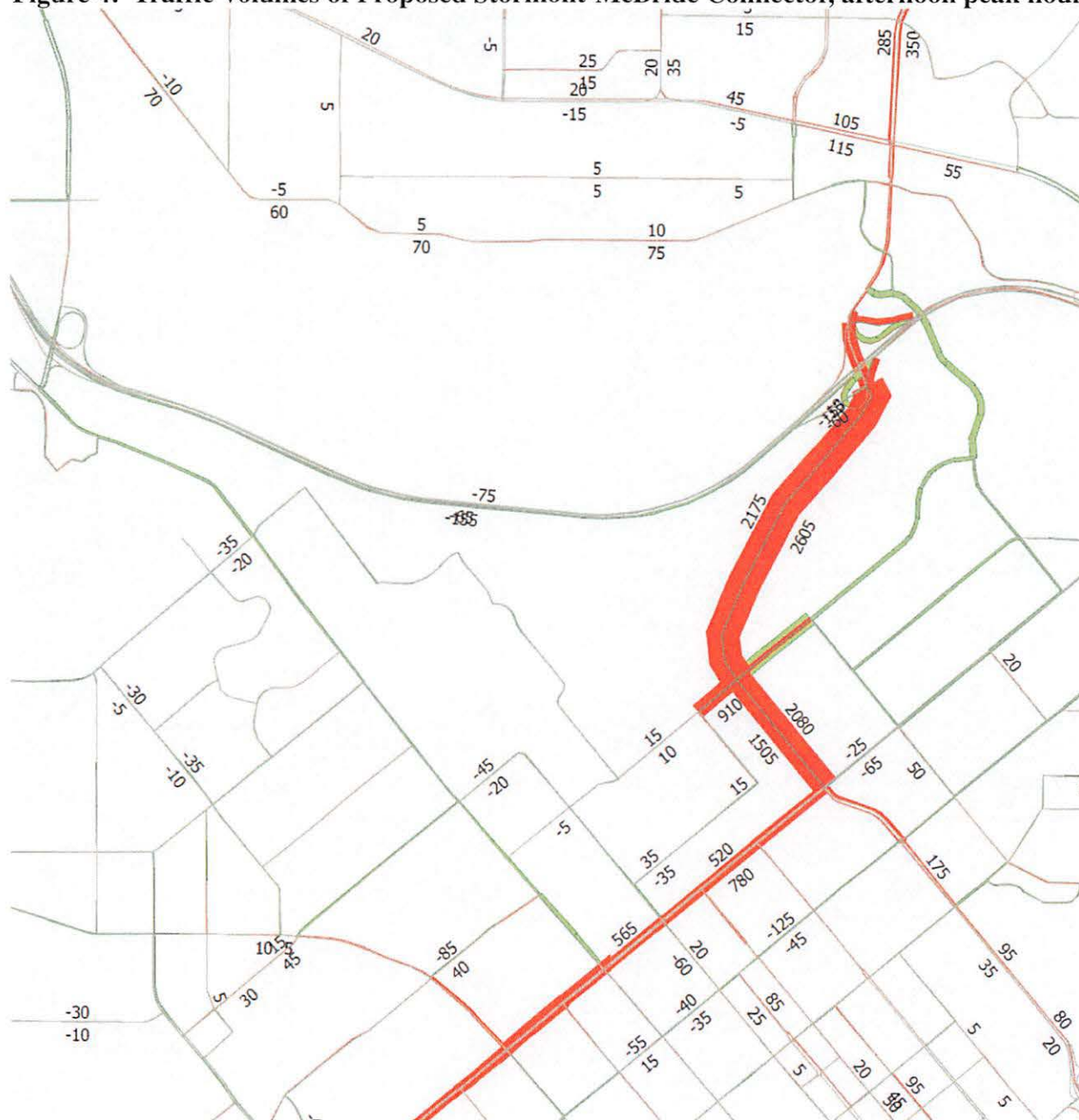
Figure 4: Traffic Volumes of Proposed Stormont-McBride Connector, afternoon peak hour
