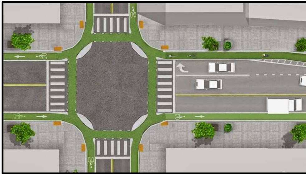
Figure 1. Example of a North American road adapted to include a protected intersection. Image credit bicycledutch.wordpress.com
