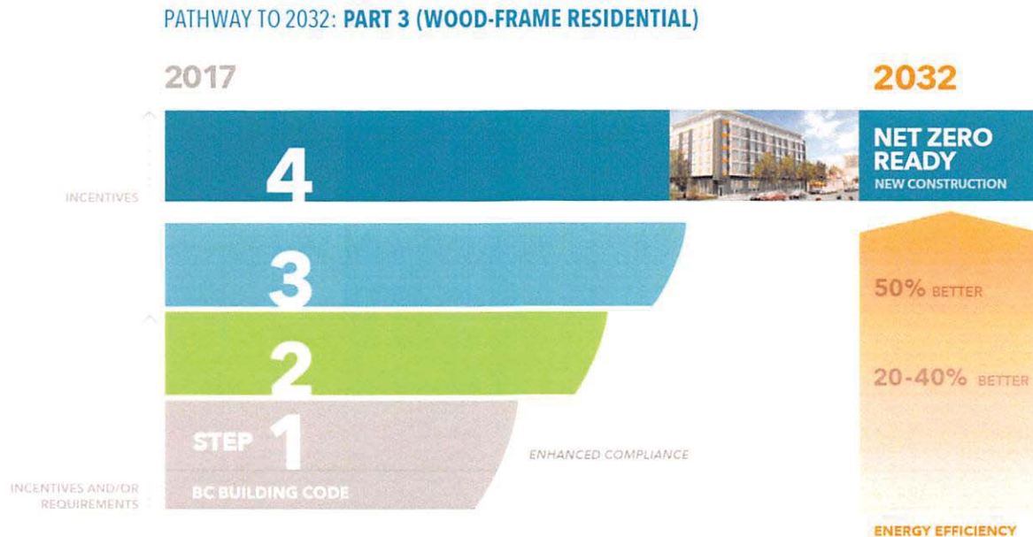
Figure 2: Steps for Part 3 wood-frame residential buildings
