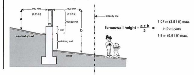
However, if a retaining wall has been constructed **on a property line**, the height of a fence or wall shall be determined by measurement from the surface of the ground that the retaining wall supports at the average grade level within 900 mm (2.95 ft.) of such retaining wall. See below.
