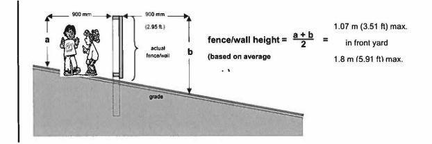
If a wall or fence has been constructed on a retaining wall, measure from the ground level at the average grade level within 900 mm (2.95 ft.) of both sides the fence or wall. See below.
