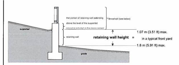
Where necessary, suitably engineered retaining walls may be combined to terrace a site. Multiple retaining walls must step back no more steeply than at a one-to-one rise to run.
