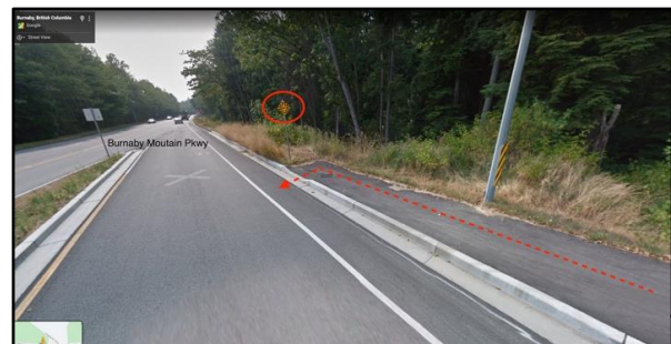
Figures 3 and 4. A bike path (red line) along the Gaglardi-Burnaby Mountain slip lane ends suddenly, requiring downhill cyclists to stop and turn 90 degrees to merge into a narrow painted bike lane.
