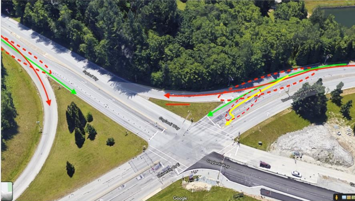
Figure 2. Right-turn slip lanes near the Gaglardi Way and Burnaby Mountain Pkwy intersection allow high-speed motor vehicles (red lines) to weave across the painted bike lanes, creating conflicts with cyclists travelling straight through (green lines). Cyclists turning left from Burnaby Mountain Pkwy onto Gaglardi Way, a typical route for SFU commuters, experience additional conflicts as they weave across two vehicle lanes to align themselves for the left turn (yellow line).
