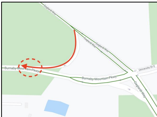
Figures 3 and 4. A bike path (red line) along the Gaglardi-Burnaby Mountain slip lane ends suddenly, requiring downhill cyclists to stop and turn 90 degrees to merge into a narrow painted bike lane.
