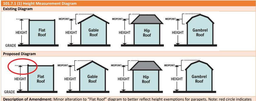
**Description of Amendment:** Minor alteration to "Flat Roof" diagram to better reflect height exemptions for parapets. Note: red circle indicate area of change, it does not form part of the amended diagram.
